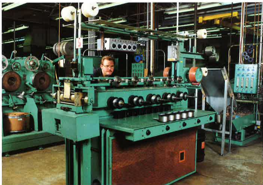
Wire is kept under tension through annealing so its speed can be carefully controlled. This enables operators to achieve more exact properties in the final product.
