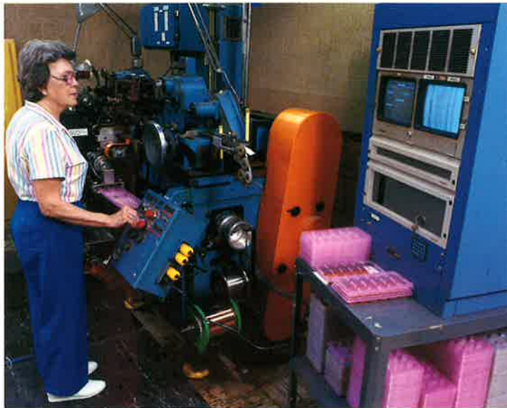
Wires are cropped, matched end-to-end, and welded in a high speed operation that produces up to 300 two and three part leads per minute.
