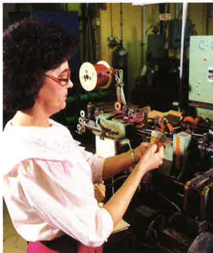
The weld area is visually inspected on every batch of leads coming off the welder.
